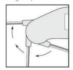
occur. It is recommended to store the probe, in the closed position, when not in use. Apply the probe to the substance to be measured. For optimum accuracy immerse at least 70 mm of the probe in the substance. **DO NOT** immerse any of the case parts in liquid. The probe should be allowed adequate time to stabilise to the temperature of the item to be measured.
